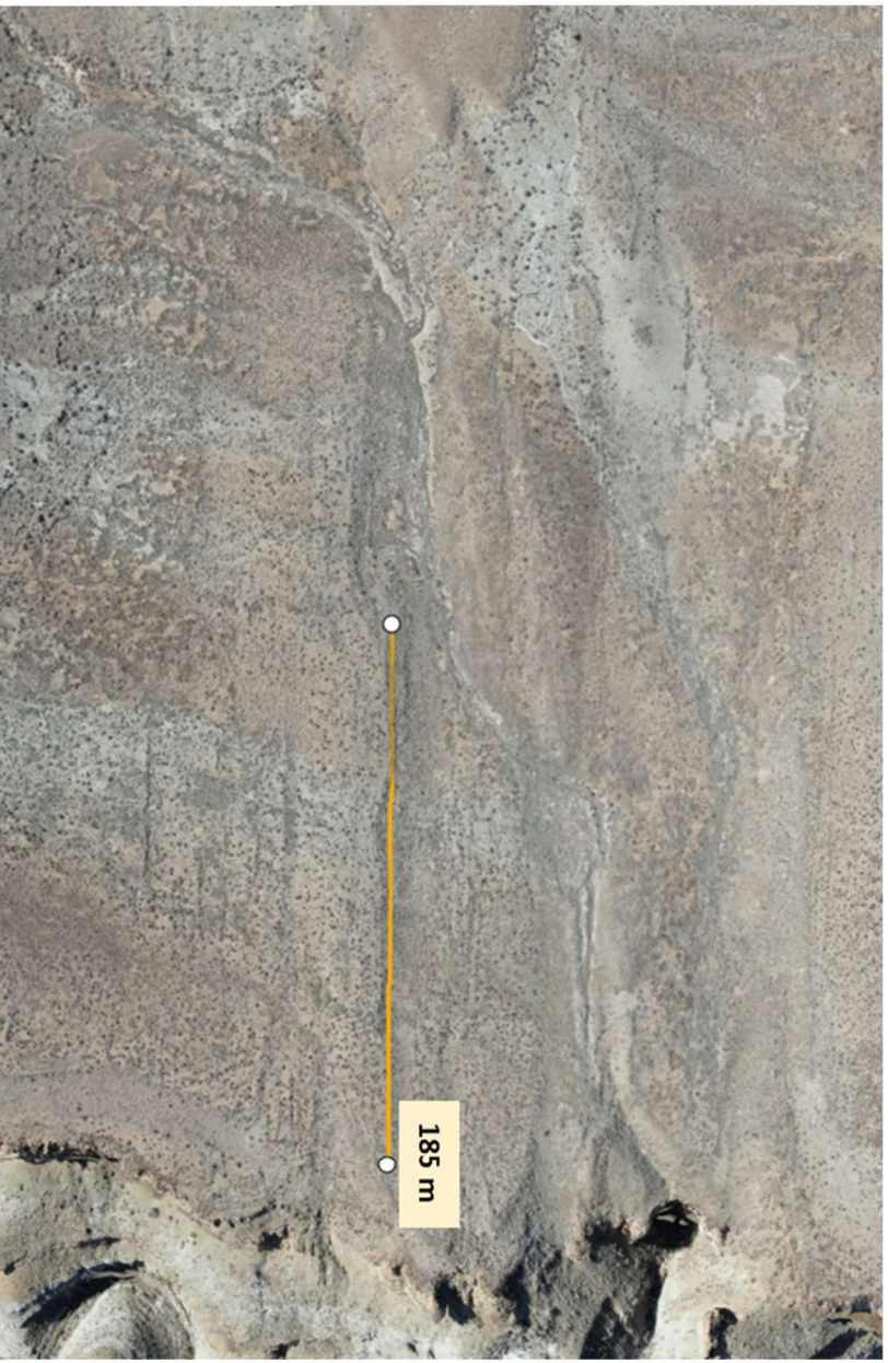
Figure 8. Plan view photo of the SWFZ as an example of methodology of the process of measuring fault length of discrete segments from drone-derived photogrammetry. Location shown in figure 4.
