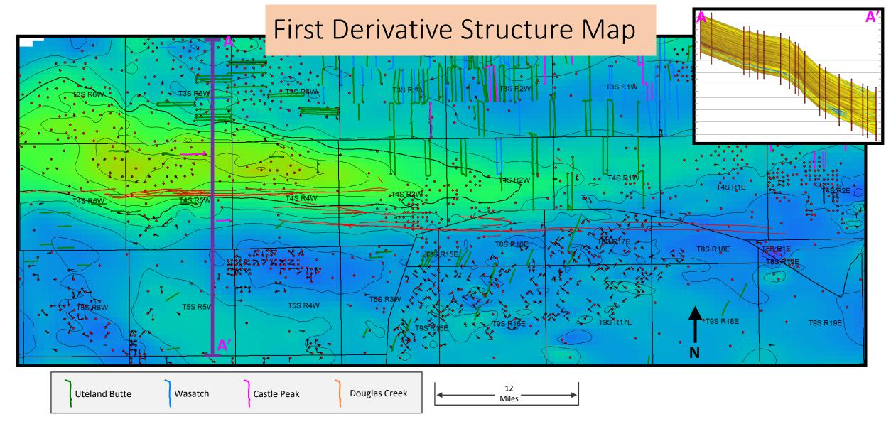
First-derivative structure contour map on the Uteland Butte member showing the portions of the basin with the steepest dips
