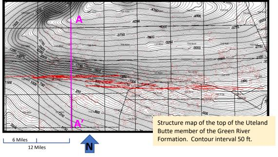
Subsea-true-vertical-depth (SSTVD) structure contour map on the top of the Uteland Butte member of the Eocene Green River Formation
