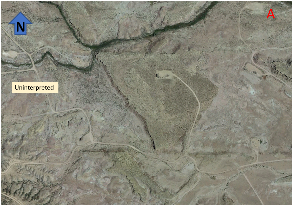
FIGURE 5: (A) Google image showing a fault segment that cuts the Eocene Uinta Formation. (A') Annotated photo shows the interpretation of right-lateral (dextral) movement along the fault segment with the offset of an exhumed channel in the Uinta Formation. The laterally offset features, called “pin points” by structural geologist, allow us to measure fault offset. This fault offset the exhumed channel ~600 ft. The roads and cleared areas are oil well pads within the Greater Monument Butte field.
